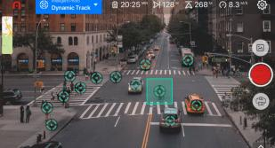
• A 3 second countdown will start automatically. After the aircraft successfully starts the tracking, the target will be surrounded by a green rectangle.
